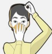
Secure ties, loops or straps and mould metal piece over nose.
